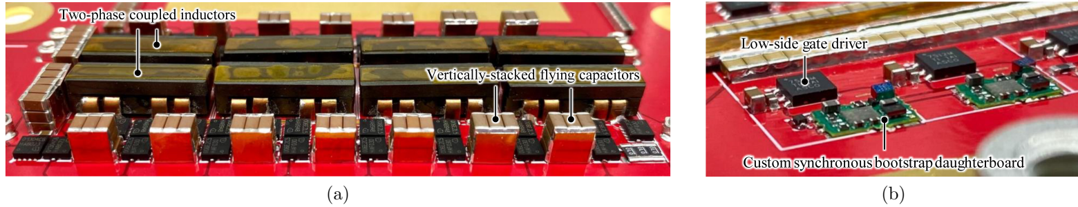
Figure 7.10: (a) Side view of the hardware prototype. (b) Photograph of the gate drive circuitry, including the custom synchronous bootstrap daughterboards (dimensions: 5.8 \times 3.5 \times 1.0 mm 3 ) used to power the high-side switches.
