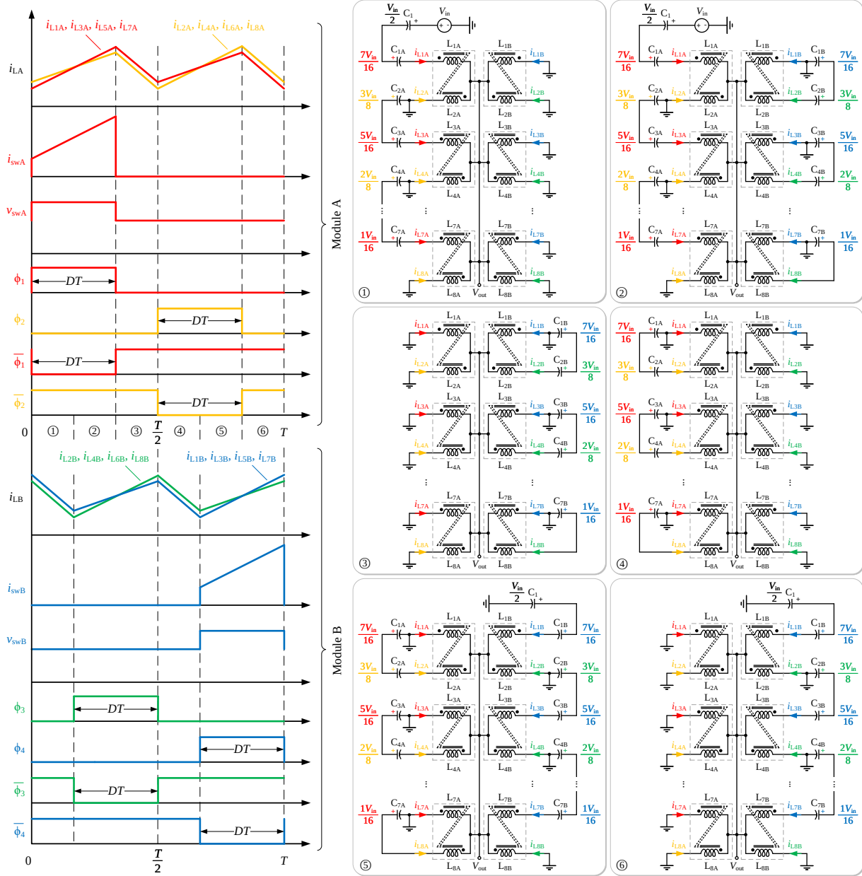
Figure 7.2: Key waveforms and control signals of the proposed switching bus converter. The equivalent circuits for the six operating modes are shown on the right-hand side. The sequence of operating modes: ① \rightarrow ② \rightarrow ③ \rightarrow ④ \rightarrow ⑤ \rightarrow ⑥ \rightarrow ① \rightarrow ② \rightarrow ③ \rightarrow \dots .
