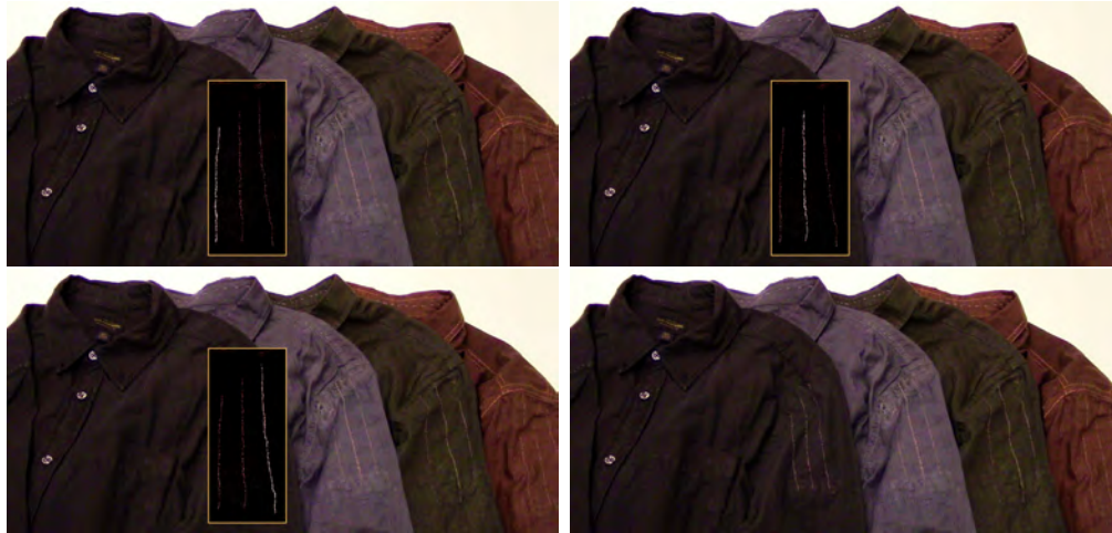
Figure 2.4: (top) Ripple, a shirt whose three shoulder pinstripes change color in response to skin conductance, was produced in multiple colors and sizes. Pinstripes fade to white one by one, then all return to gray (left to right, top to bottom) .
