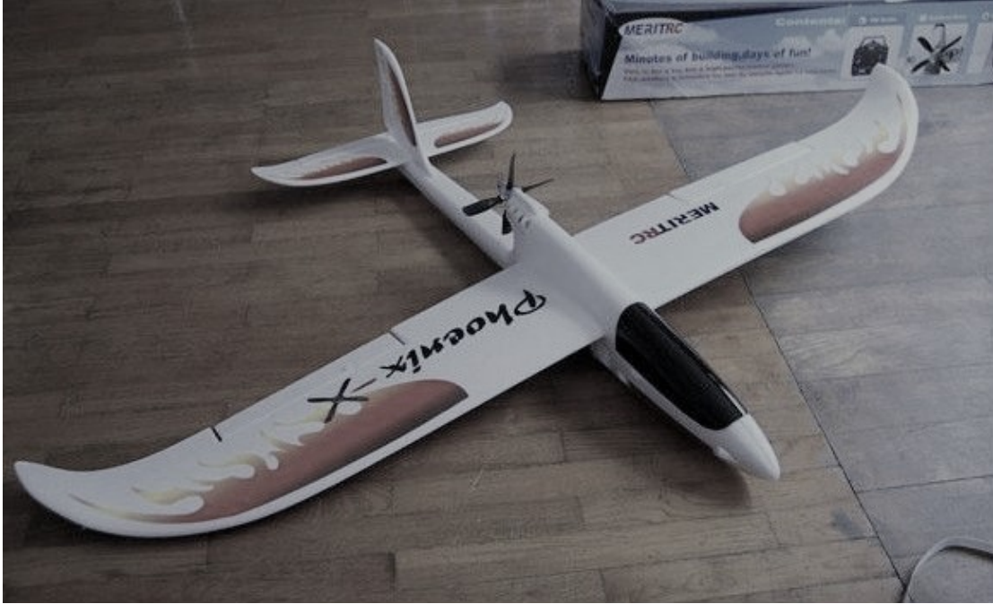
Figure 5.1: RC model plane - EPO glider phoenix 1370mm.
