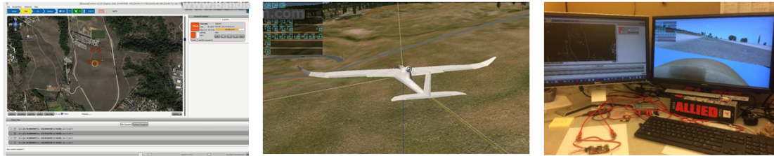
Figure 5.9: MHIL test setup is shown. On the left, QGC software runs on a separate PC. In the middle, X-Plane simulator software runs on a separate PC and communicates with the QGC software and AUAV3 through a serial link. On the right AUAV3 runs the test autopilot software version and is connected through a serial port to the PC.
