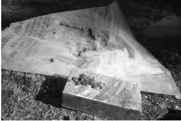
Figure 5.3. Polishing device (fire brick) with polishing matrix (sand containing silicates).
