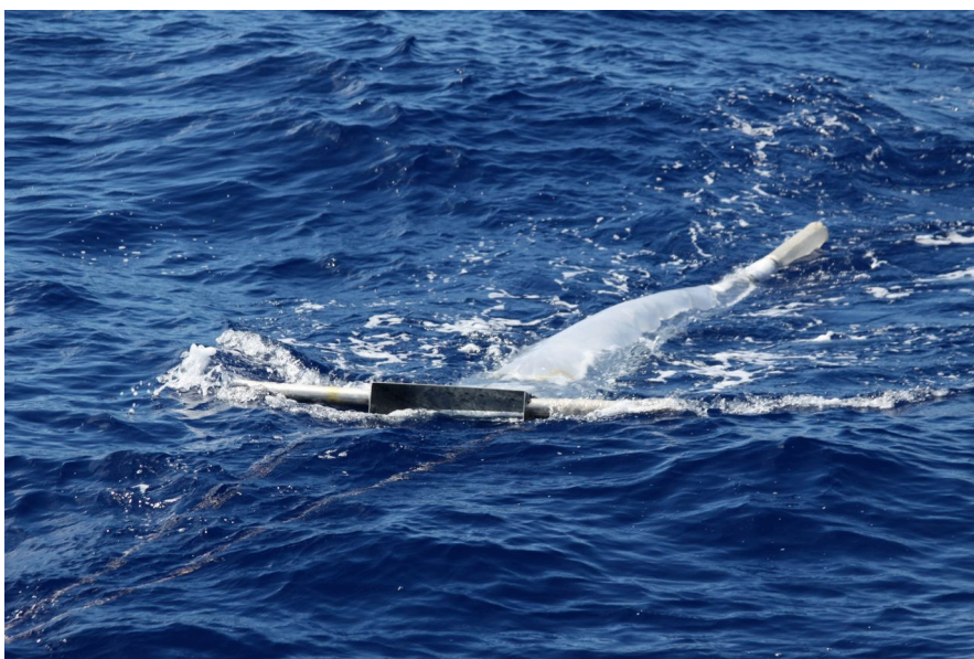
Figure 4.1: The 'suitcase' manta trawl. Photo courtesy Rob Johnson.
