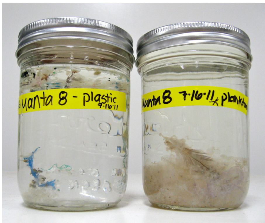
Figure 5.3: Ocean surface sample sorted into plastic and plankton at the University of Hawaii Hilo. Photo by the author.
