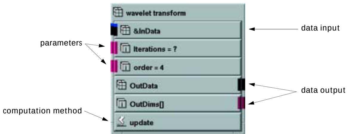
Figure A.1 AVS/Express module for the B-spline wavelet transform component. Different data types are color-coded.
