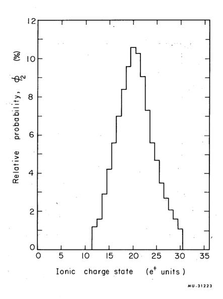
Fig. 6. Charge-spectrum histogram. Relative probability  $\varphi_{\rm Z}$  (%) as a function of ionic charge state of nuclear reaction product. Target thickness: 9.7  $\mu g/cm^2$ .
