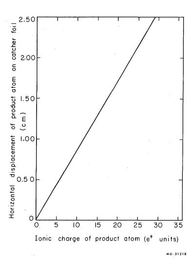
Fig. 1. Horizontal displacement of product atom on catcher foil, in cm, as a function of the ionic charge of the reaction product according to Eq. (1) for  $A_1=149$ ,  $\langle v \rangle = 4.5 \times 10^8$  cm/sec, H = 3150 gauss, t=15.2 cm, and L = 5.3 cm. (The symbols are explained in the text.)
