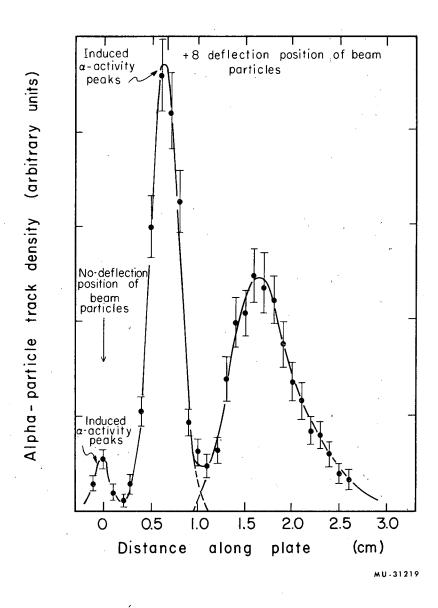
Fig. 2. Experimental scanning curve. The horizontal displacement of particles on the catcher foil (D) equals the distance along the plate as a function of the  $\alpha$ -particle track density. The target thickness is 9.7  $\mu g/cm^2$ . (The experimental conditions are described in the text).
