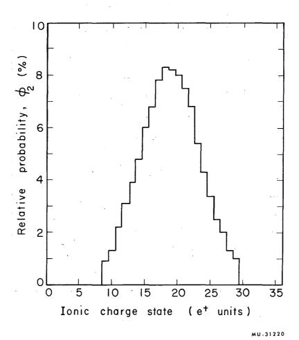
Fig. 3. Charge-spectrum histogram. Relative probability  $\varphi_z$  (%) as a function of the ionic charge state of the nuclear-reaction product. Target thickness: 26.2  $\mu g/cm^2$ .
