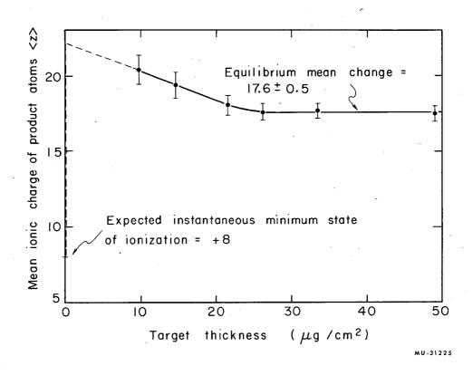
Fig. 8. Mean ionic charge of the product atom as a function of target thickness. The equilibrium mean charge is  $17.6 \pm 0.5$ . 9, 10
