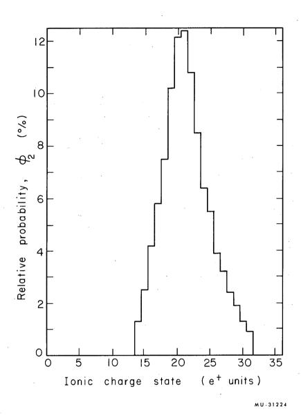
Fig. 7. Charge-spectrum histogram for zero target thickness obtained by linear extrapolation for the various charge-state probabilities to zero target thickness.
