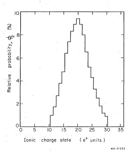
Fig. 5. Charge-spectrum histogram. Relative probability  $\varphi_{Z}$  (%) as a function of ionic charge state of nuclear reaction product. Target thickness: 14.6  $\mu g/cm^{2}.$
