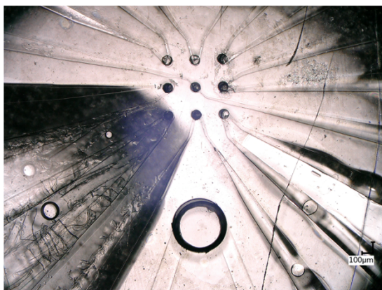
Figure 45 Hydrogels that swell too much break SU8 channels.
