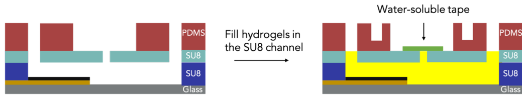
Figure 39 Fabrication of hydrogel in the vertical ion pump.
