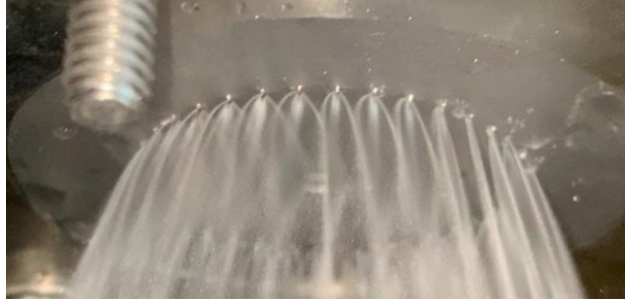
Figure 2.4: Image of simultaneous cold-flow testing of the fuel and oxidizer flow paths for the unhoneed additively-manufactured injector using water.
