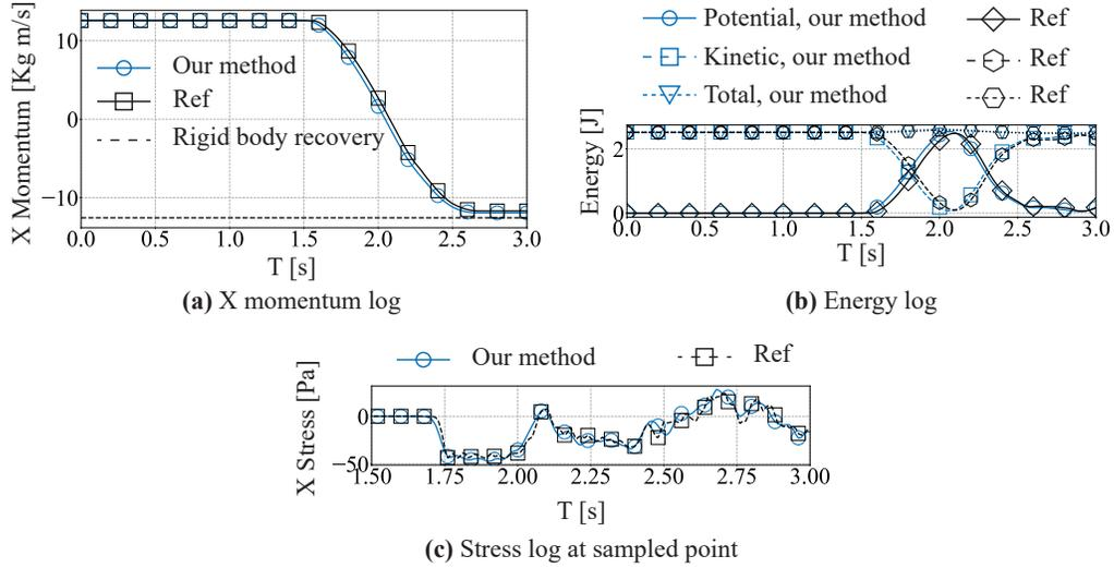
Figure 2.15: System momentum, energy, and sampled stress of the 2D collision disks. (a) The momentum in the  $x$ -direction of the left disk, (b) the energies of the system, and (c) the stress at the sampled particle closest to the center of the left disk.
