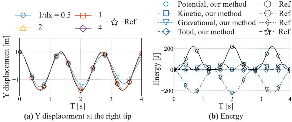
Figure 2.17: Displacements and system energy of the 2D cantilever without rotation. Plots of (a) the displacement in the  $y$ -direction at the right tip of the cantilever and (b) the energies of the system.
