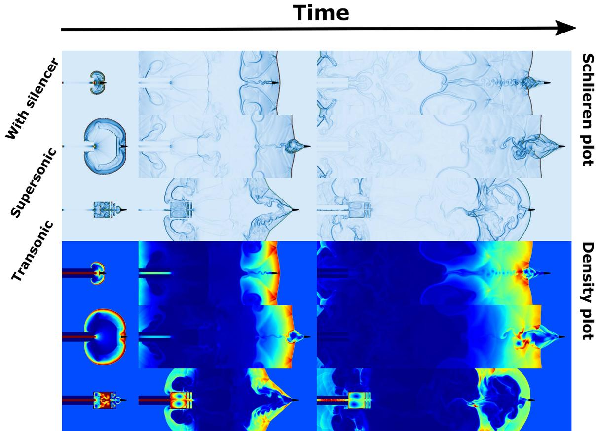
Figure 3.12: Demo: 2D Bullet simulations. Schlieren & density plots depicting the firing of heavy (left,  $\rho = 1250kg/m^3$ ) and light (middle,  $\rho = 500kg/m^3$ ) bullets, along with a light bullet equipped with a silencer at the chamber outlet (right,  $\rho = 500kg/m^3$ ). Snapshots are captured at intervals of 0.028s, 0.0935s, and 0.17s, from bottom to top.
