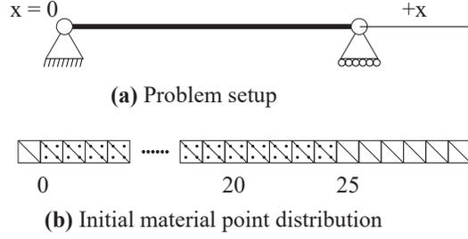
Figure 2.11: Setup of the 1D bar vibration test.
