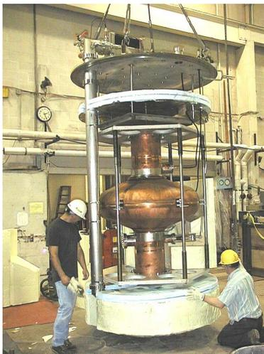
Figure 10: 201 MHz superconducting cavity under test at Cornell.
