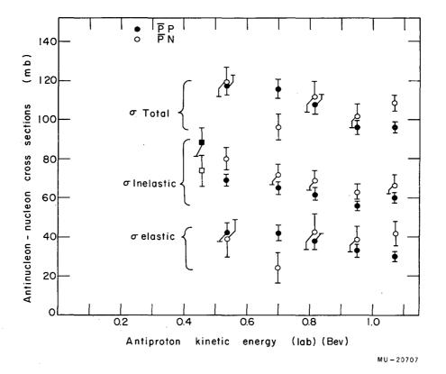
Fig. 16. Comparison of  $\overline{p}$ -p and  $\overline{p}$ -n cross sections in the energy range 450 to 1068 Mev.
