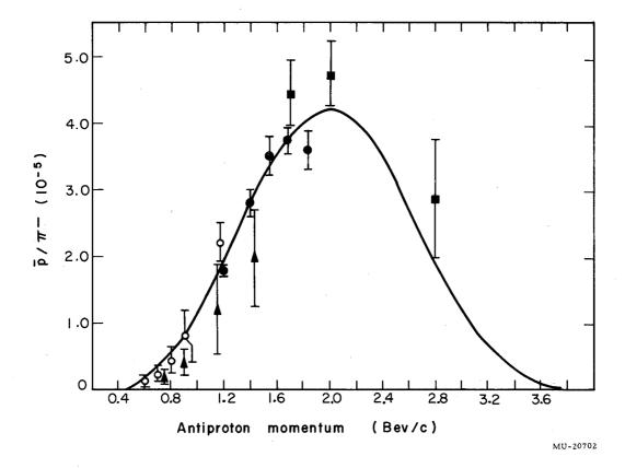
Fig. 10. Momentum distribution for antiprotons produced by approx 6-Bev protons on carbon and beryllium. The experimental points are taken from Table II. The curve is calculated by a statistical model.
