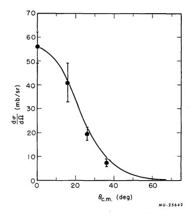
Fig. 11. Angular distribution of  $\overline{p}$ -p elastic scattering at 534 Mev.
