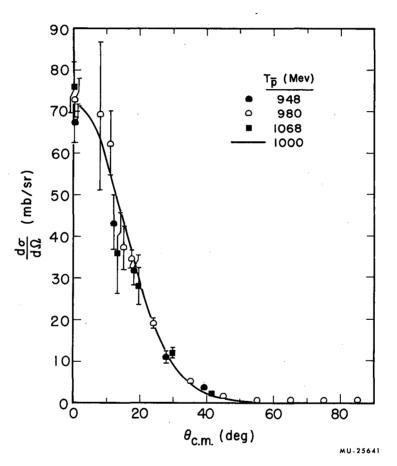
Fig. 13. Angular distribution of  $\overline{p}$ -p elastic scattering near 1 Bev. The 980-Mev points are from Armenteros et al. (reference 24).
