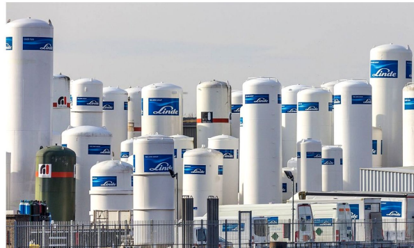
Figure 18: Horizontal and vertical LH2 storage
