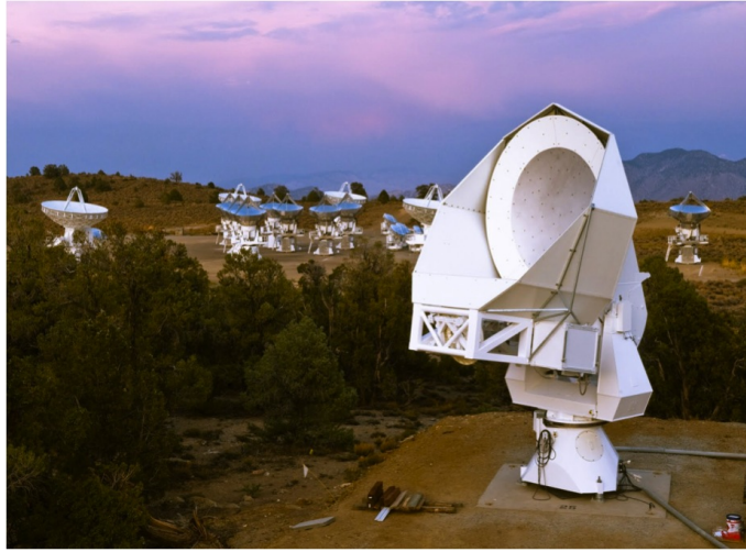
Figure 5.1: POLARBEAR-I on the Huan Tran Telescope at the Cedar Flat engineering site. The telescope was seated on a foundation pad borrowed from the CARMA array, which can be seen in the background. Photo credit: Huan Tran
