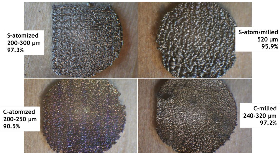
Figure 9. Comparison of atomized and milled particle laser coalesced layer thickness and Archimedes densities. All cases were coalesced with 12W, 82.5 mm/s, and 50 μm hatch.
