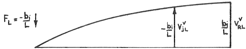
Fig. 17b LOAD APPLIED AT L
