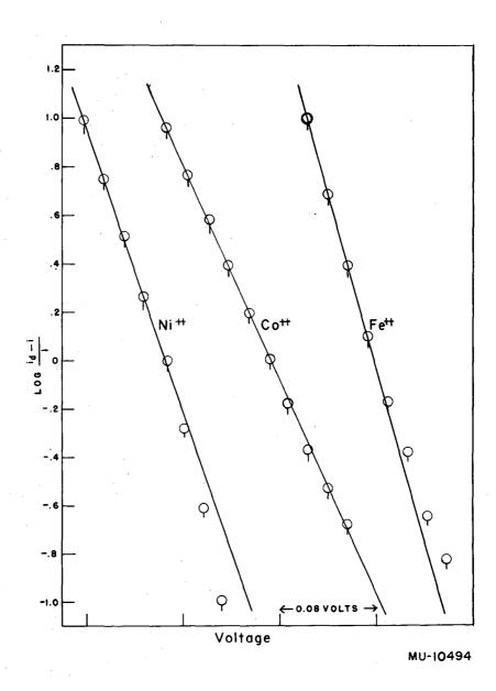
Fig. 7. Log (i<sub>d</sub> - i)/i vs. potential plot for nickelous, cobaltous and ferrous ions at 25.0 °C. in 0.1 M NaCl. The plots apply to the current-voltage curves in Fig. 4.
