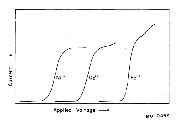
Fig. 5. Typical current-voltage curves for the reduction of nickelous, cobaltous and ferrous ions at 25.0 °C. in 0.1 M NaClO<sub>4</sub> and 0.01% agar.
