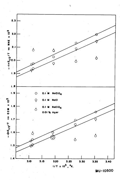
Fig. 13. Plots of  $-anE_{1/2}/T$  vs. 1/T for cobaltous ion.
