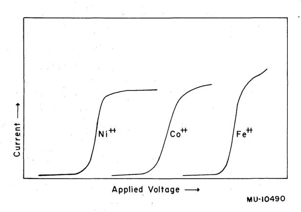
Fig. 3. Typical current-voltage curves for the reduction of nickelous, cobaltous and ferrous ions at 25.0 °C. in 0.1 M NaClO<sub>4</sub>.
