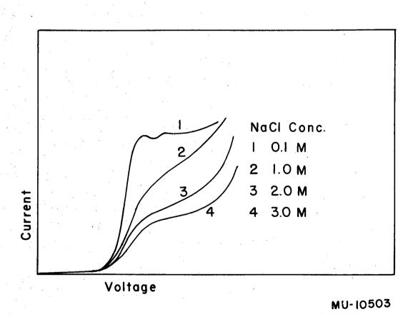
Fig. 16. Current-voltage curves of ca. 1 mmolar nickel in NaCl solutions, pH 3.
