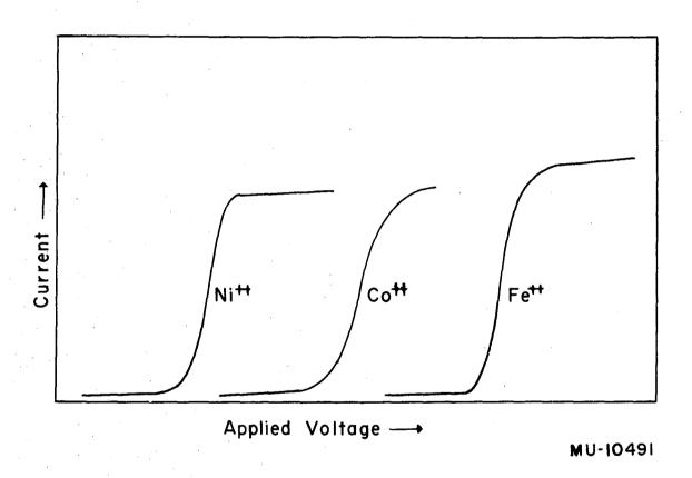
Fig. 4. Typical current-voltage curves for the reduction of nickelous, cobaltous and ferrous ions at 25.0 °C. in 0.1 M NaCl.
