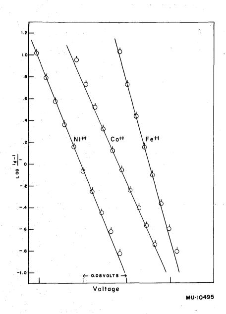
Fig. 8. Log (i<sub>d</sub> - i)/i vs. potential plot for nickelous, cobaltous and ferrous ions at 25.0 °C. in 0.1 M NaClO<sub>4</sub> and 0.01% agar. The plots apply to the current-voltage curves in Fig. 5.
