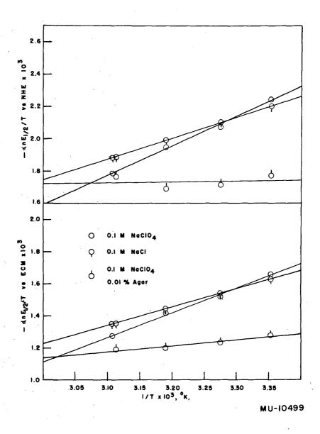
Fig. 12. Plots of  $-anE_{1/2}/T$  vs. 1/T for nickelous ion.
