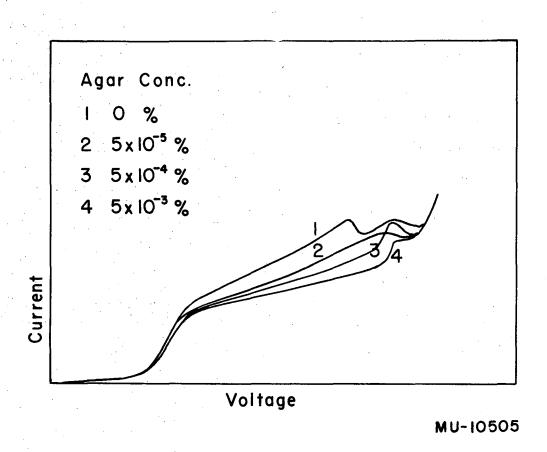
Fig. 18. The effect of agar on the current-voltage curves of ca. 0.8 mmolar nickel in 3.0  $\underline{\text{M}}$  NaClO<sub>4</sub>.
