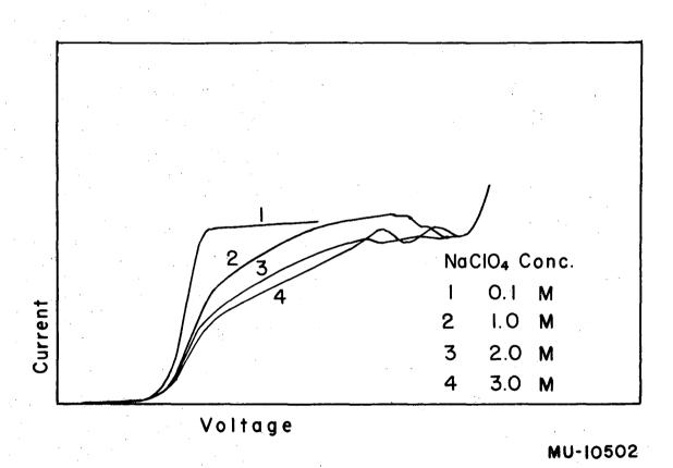
Fig. 15. Current-voltage curves of ca. 0.8 mmolar nickel in NaClO<sub>4</sub> solutions.
