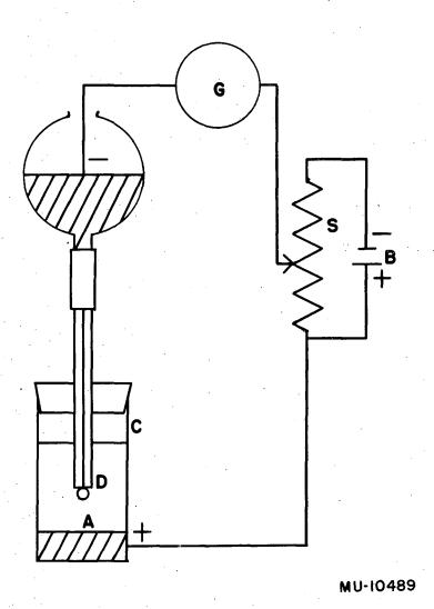
Fig. 2. A simple polarographic circuit.
