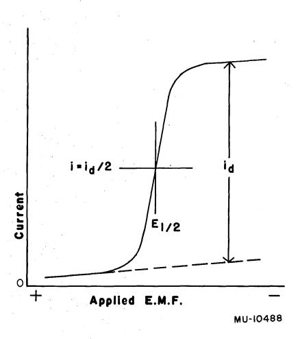
Fig. 1. A typical current-voltage curve.
