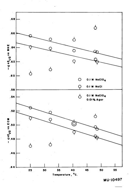
Fig. 10. Plots of -anE<sub>1/2</sub> vs. temperature for cobaltous ion.
