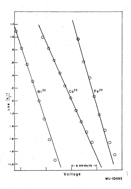
Fig. 6. Log (i<sub>d</sub> - i)/i vs. potential plot for nickelous, cobaltous and ferrous ions at 25.0 °C. in 0.1 M NaClO<sub>4</sub>. The plots apply to the current-voltage curves in Fig. 3.
