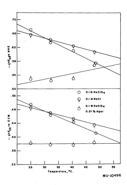
Fig. 9. Plots of -anE<sub>1/2</sub> vs. temperature for nickelous ion.
