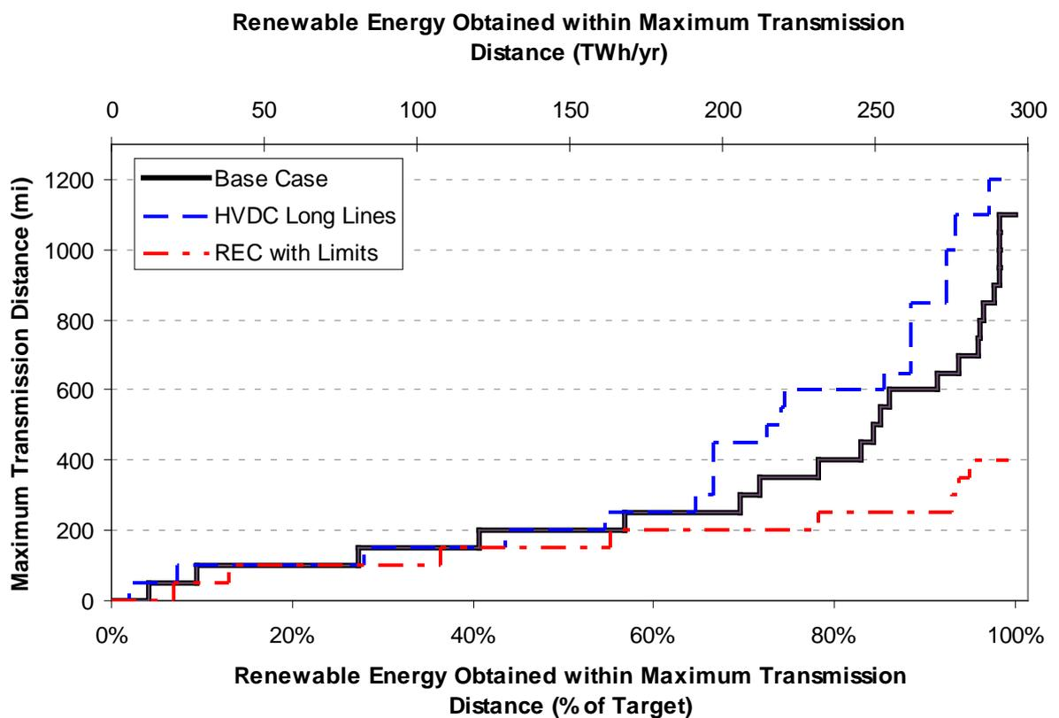
*Note: Each step increases the maximum transmission distance by 50 miles.*
