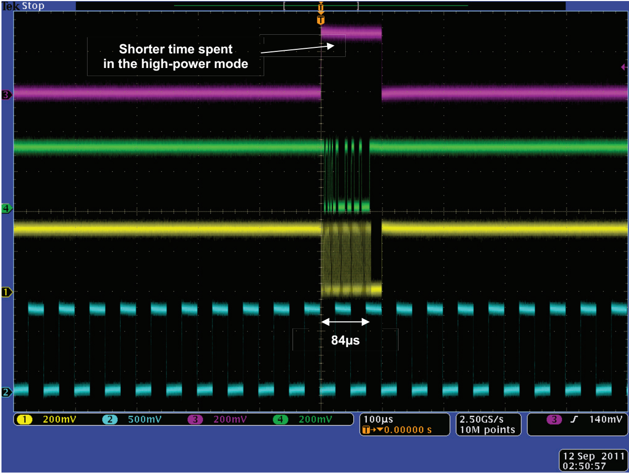
Figure 5.12: Dynamic behavior of asynchronous processor at 0.3V.
