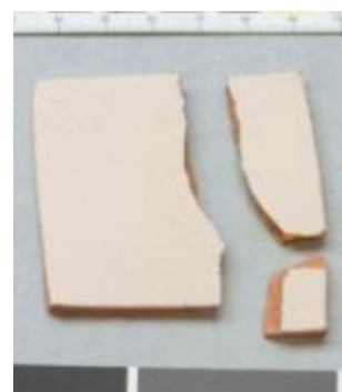
Sodium Hydroxide tile AT
