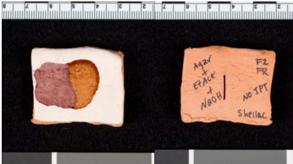
1:1 Ethanol and acetone in agar and NaOH – applied as a warm soft gel at pH 13.5 w/o intermediary layer (Top and Bottom views)
