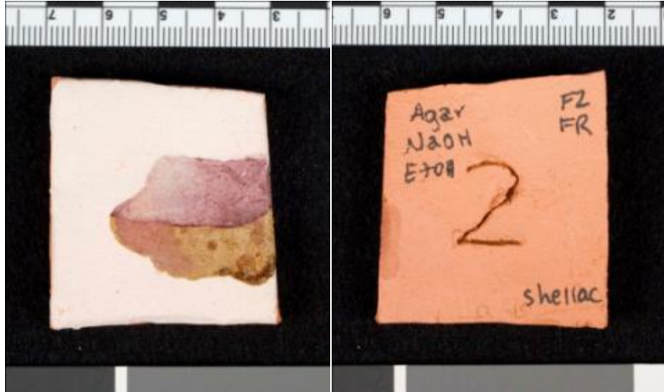
Ethanol in agar and NaOH – applied as a warm soft gel at pH 13.5 w/o an intermediary layer (Top and Bottom View)
