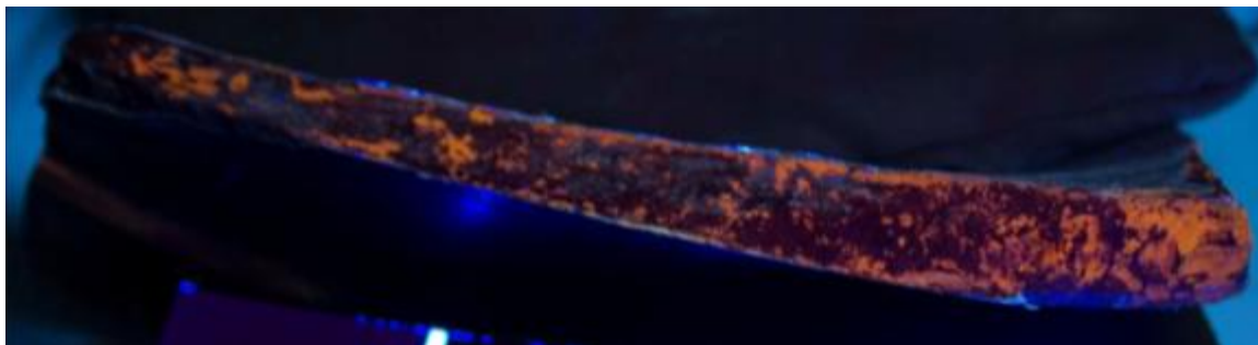
UV-Visible fluorescence photograph of fragment after treatment. Long-wave ultraviolet light was used to excite the shellac (in orange). The image was captured using an unmodified DSLR with a visible-pass filter (400-700nm with some leaks in the IR range).
