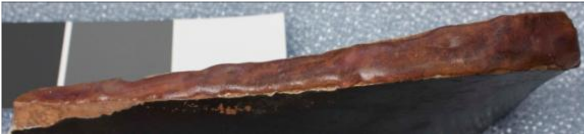
Treatment application 1: pH = 13.5 Time Elapsed = 5 minutes
