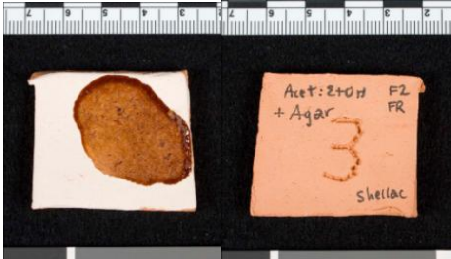
1:1 Ethanol and acetone in agar – applied as a warm soft gel at pH 7.5 w/o an intermediary layer (Top and Bottom View)
