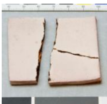
Ammonium Hydroxide tile AT
