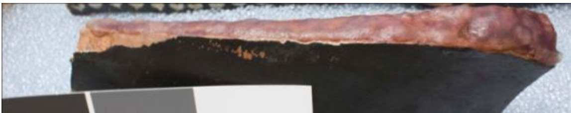
During treatment application 3; pH = 13.5 Time Elapsed = 5 minutes
