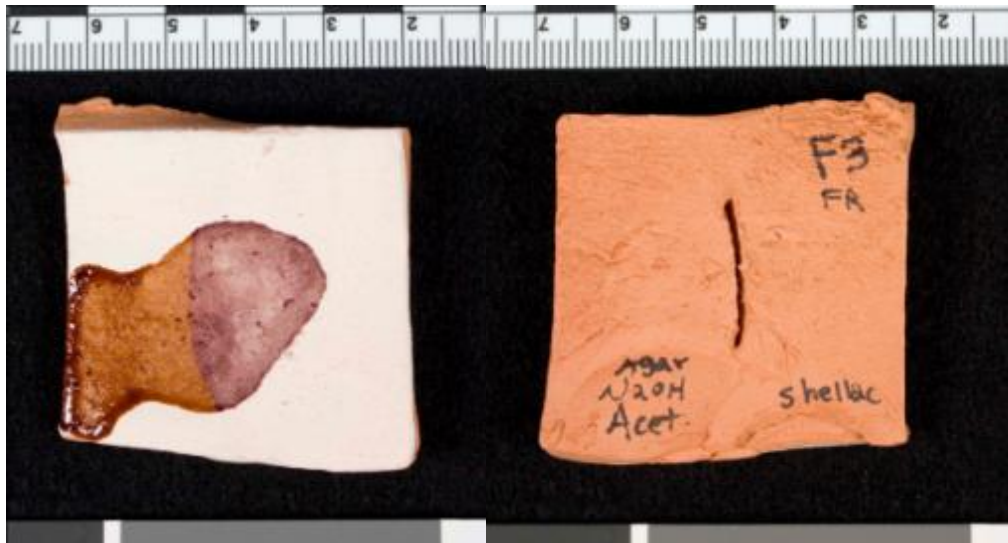
Acetone in agar and NaOH – applied as a warm soft gel at pH 13.5 w/o an intermediary layer (Top and Bottom View)
