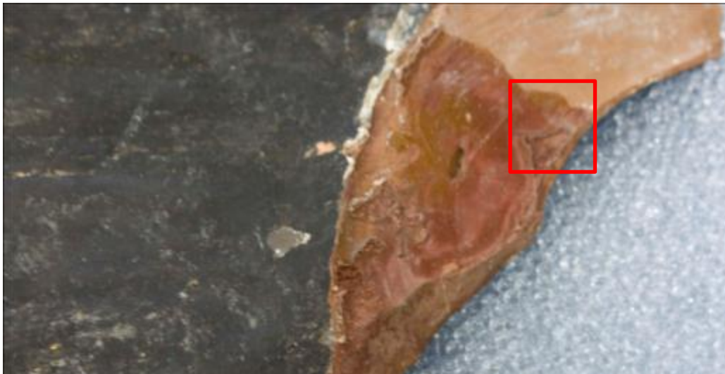
Detail of area to be treated (shown in red box in above image). The treatment used employed NaOH in warm soft gelled agar with a Japanese tissue paper intermediary layer. pH = 10.5
