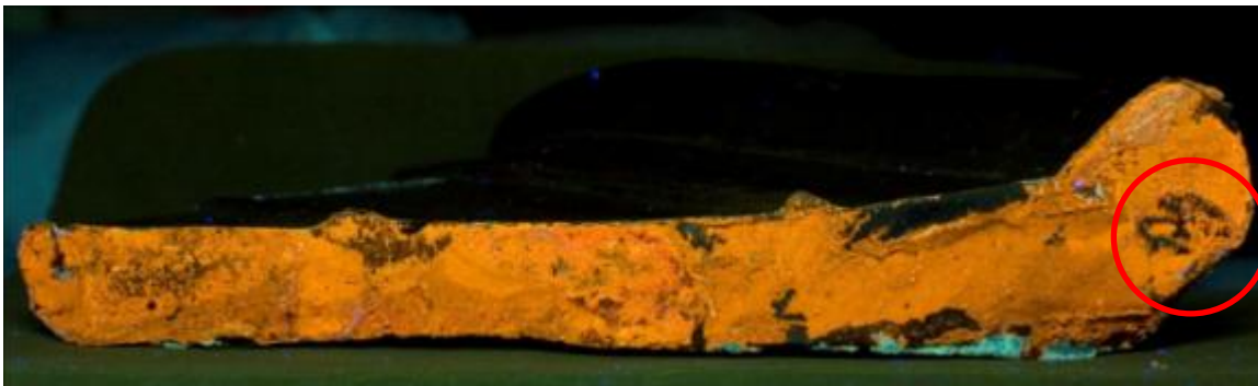
Rim fragment used in Trial 9 BT using Long wave Ultraviolet-visible fluorescence. Orange indicates the presence of shellac. It is possible to see areas of shellac removal from Trial 8 (indicated above).
