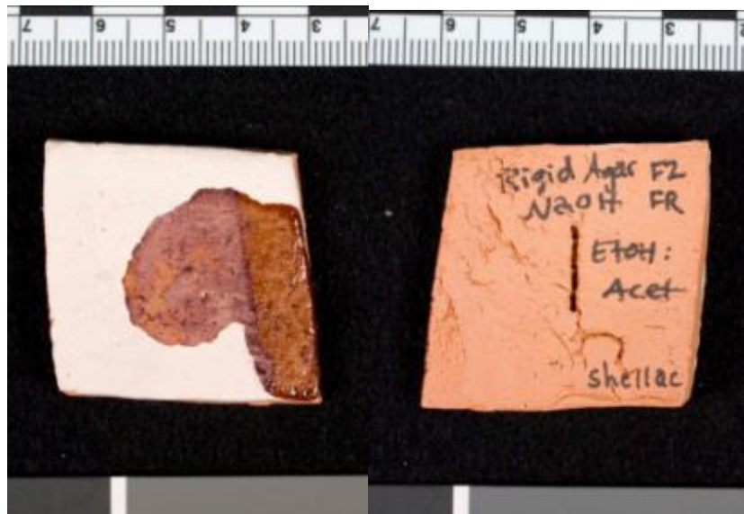
1:1 Ethanol and acetone in agar and NaOH – applied as cooled rigid gel w/o intermediary layer at pH 13.5 w/o an intermediary layer (Top and Bottom View)
