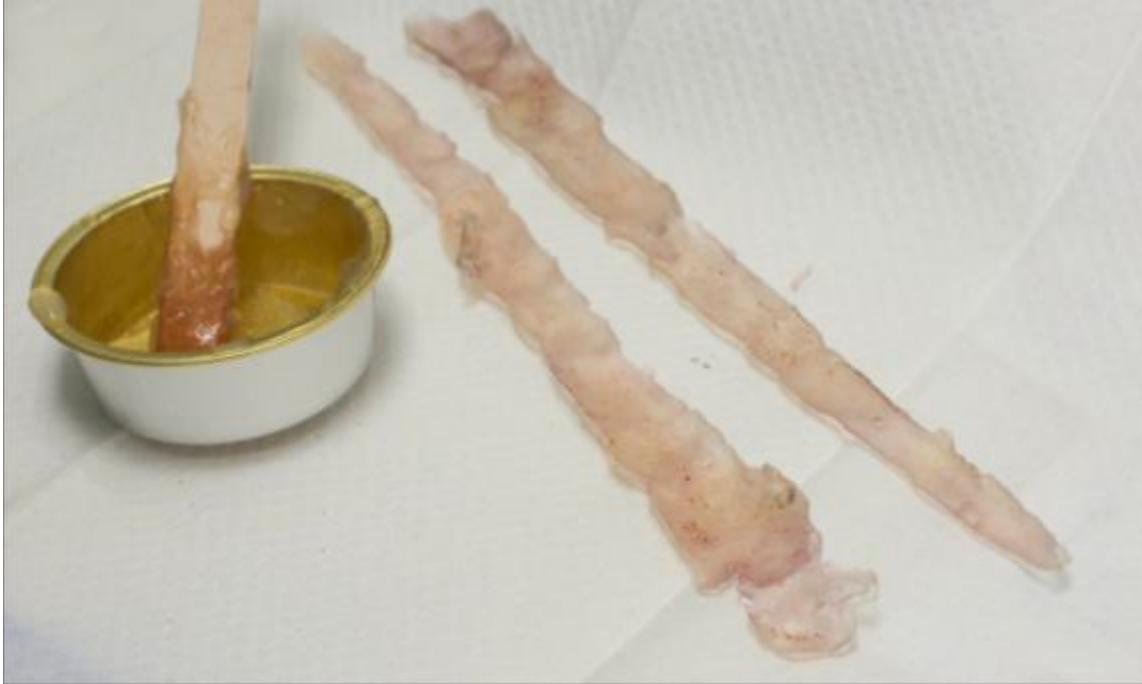
Figure 13: Agar poulitices after removal from shellac coated edges (from Trial 10) showing the lac dye and other small particulate matter from the fragment edge having been drawn into the gel matrix (lending the gel a pinkish color).
