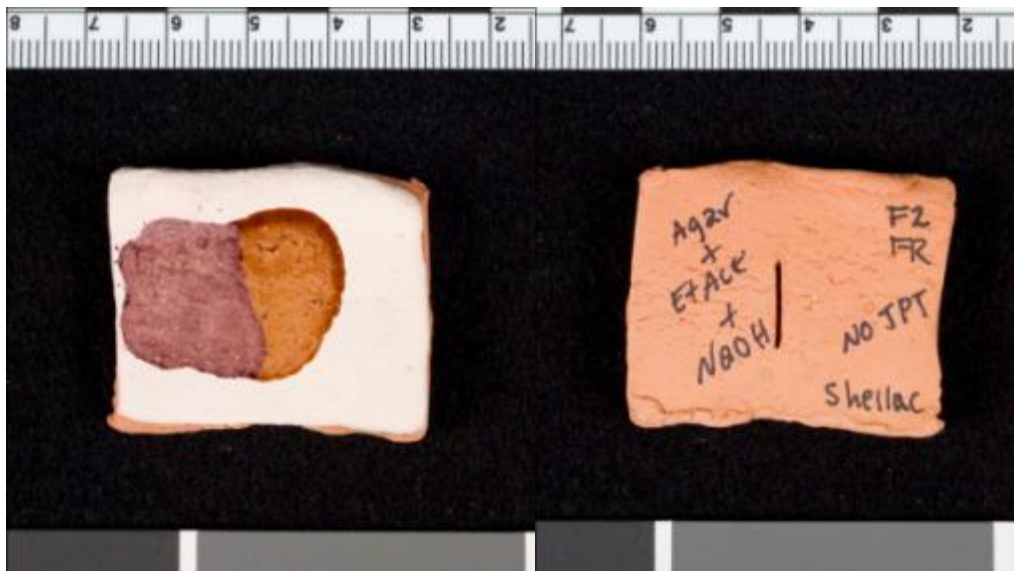
1:1 Ethanol and acetone in agar and NaOH – applied as a warm soft gel at pH 13.5 w/o intermediary layer (Top and Bottom views)
