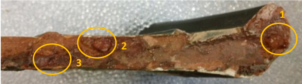
Rim fragment during treatment – after removal of third application. Total time elapsed = 40 minutes
