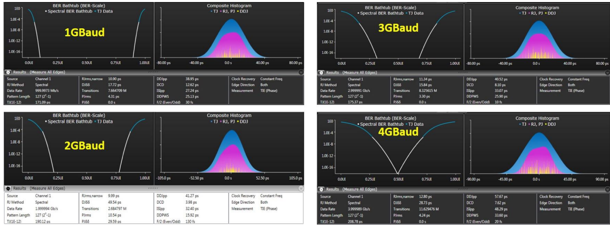
Figure 7.21: Bathtub curves, and timing jitter data captured in Keysight oscilloscope DSAV134A for 1, 2, 3, and 4 GBaud data rate QPSK data transmission over 25 cm wireless link at 146.7 GHz carrier frequency.
