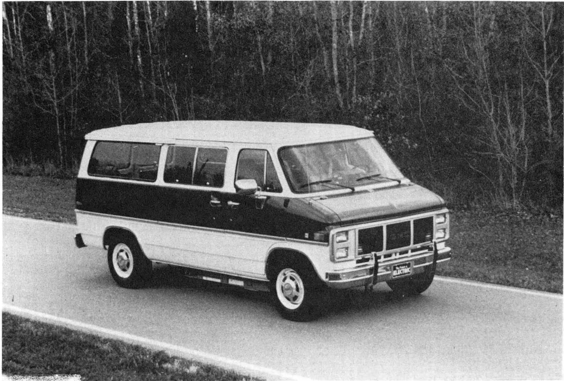
Figure 4. The G-van proof-of-concept electric vehicle. (CBB 8811-11141)
