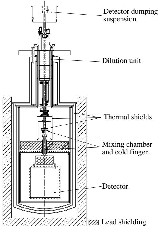
Fig. 9. CUORE cryostat and shielding.
