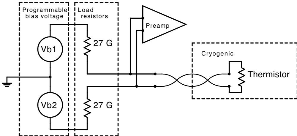
Fig. 10. Functional block diagram of the front-end electronics. Normally  $R_L$  is  $27\text{ G}\Omega$ . For determination of a bolometer I-V characteristic a command from the computer can reduce  $R_L$  to  $5.5\text{ G}\Omega$ .
