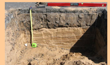
Test pit - note variable layer thickness
