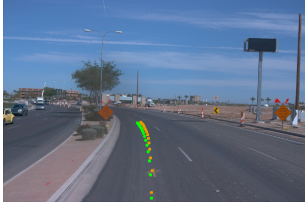
Figure 4.5: An example of the ground-truth future waypoints (green) and waypoints predicted by our model (orange). The predictions are for 1.6s into the future after the last frame in the input sequence.
