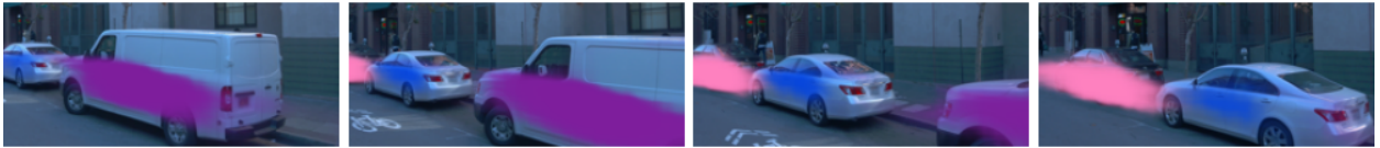
Figure 4.3: Our model is able to track many vehicles and pedestrians in held-out validation runs from the real-world Waymo Open dataset. We use Hungarian matching to determine best-fit predicted masks for each ground-truth object as described in section 4.4. In this figure, the alpha-value of the colored mask pixels is determined by the weight of the mask at each pixel.
