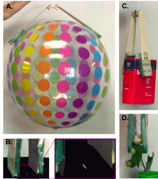
Fig. 30. A sampling of objects that the lateral shear gripper can lift. A) A 1 m diameter ball. B) A 1 mm diameter pin. Inset at right shows magnified view. C) A 3.4 kg book. D) A flower. Note that the same preload, supplied only by the weight of the arms is used to lift both heavy and delicate objects.
