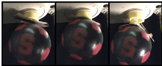
Fig. 29. Curved surface gripper passively catching a ball thrown at it.
