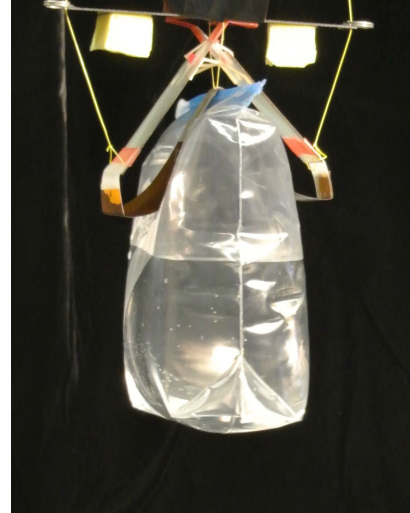
Fig. 1. A flexible shear-activated gripper holds a water-filled bag. Load tendon is at center; outer tendons release the adhesive film.
