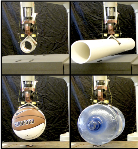
Fig. 28. Grasping tasks with a curved surface gripper implemented on a robotic arm. The gripper is shown lifting (clockwise from upper left): packing tape, 3.5 kg PVC tubing, empty 5-gal water jug, and a regulation basketball.
