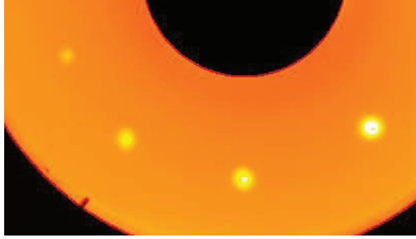
Figure 5.2: SRA image of four spreading droplets on a smooth CNx disk surface.
