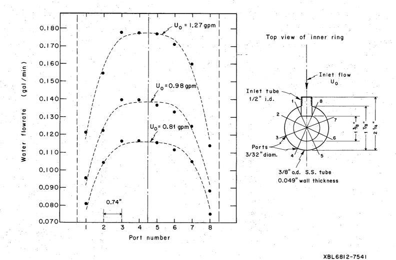
Fig. 17. Flow distribution around a jetting ring.
