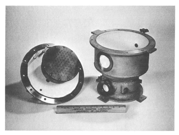
Fig. 12. Column head and flange plate.
