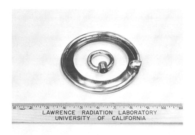
Fig. 21. Addition of brass bonnet to outer intake ring.
