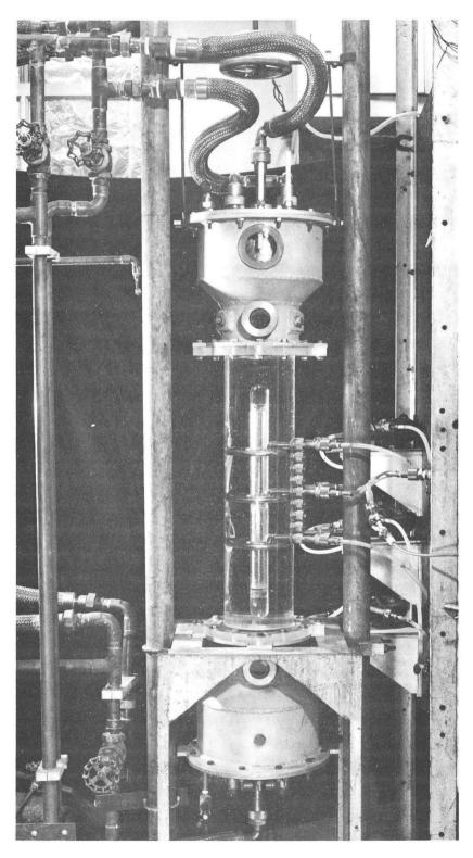
Fig. 19. Completed column assembly with central cylindrical wall.
