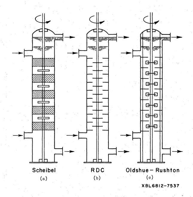
Fig. 1. Mechanically-aided column-type extractors (adapted from Ref. 1).
