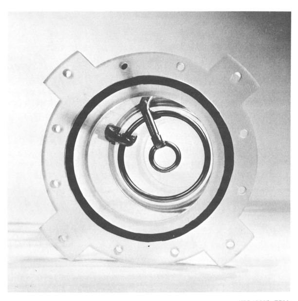
Fig. 15. Top view of a ring stage.
