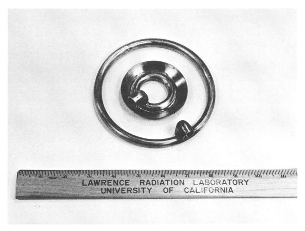
Fig. 22. Addition of brass bonnet to inner intake ring.
