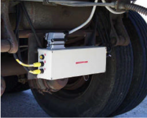
(c) Brake control circuit box
