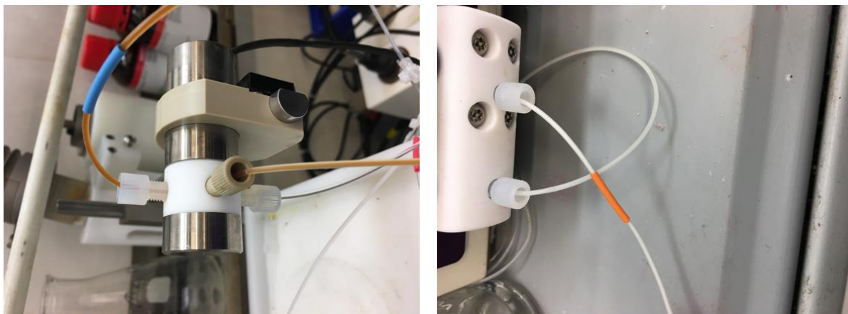
Figure 8: Filtering of NPs in line at switching valves and 90° turns (left) and crystallization of organic product in line at BPR (right)
