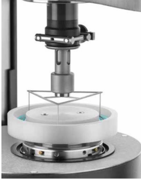
Figure 2.7: Rheometer and the double wall ring. The photo is adapted from TA instrument website
