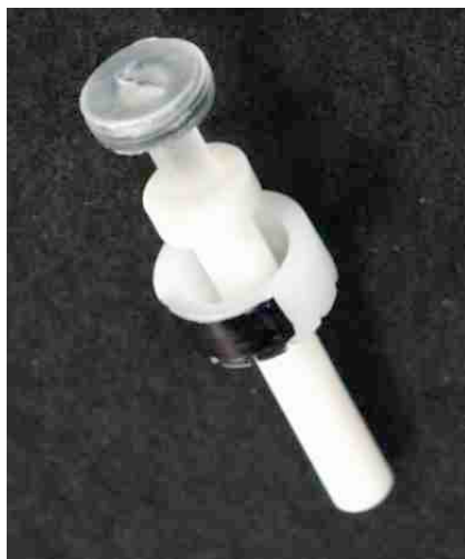
Figure 2.2 Photograph of an HR-MAS rotor. The rotors consisted of a T-shaped zirconium base, a plastic collar with machined grooves on the underside, and an opaque plastic insert fitted with a rubber O-ring and a threaded head. The insert mated with the plastic collar and provided a leak proof seal for the rotor. The grooves in the collar served as a turbine and caused the rotor to spin when air was blown across it (40).
