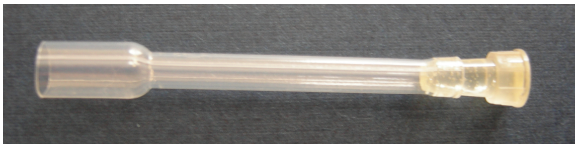
Figure 4.8 A photograph of a sample tube designed for storing tissue cultures. The sample tube was fabricated from a plastic transfer pipette.
