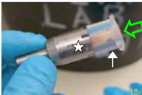
Figure 4.7 Photograph of prostate tissue core ( Green Open Arrow ) after it has been embedded in agarose gel ( White Solid Arrow ) to attach it to a stainless steel microtome plunger ( White Star ).
