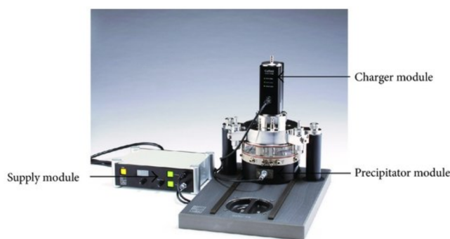
Figure i: Cultex RFS Exposure System
