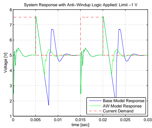
Figure 3.4: System Response with -1 V Anti-Integral Windup Limit
