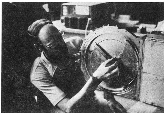
Fig. 20. Graduate student Jim Welch inserting a filament ion source on the 12-inch cyclotrino. The cyclotrino has one "dee" visible behind Jim's hand. The gap is vertical, and the entire instrument slides between the pole tips of the NMR magnet visible behind Jim.
