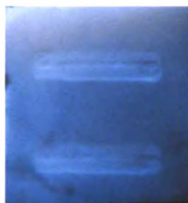
Figure 4 - A digital photograph of a bovine enamel block irradiated with two parallel Er:YAG laser cuts.
