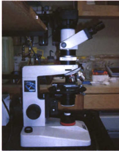
Figure 10 - Light microscope used for polarized light microscopy. A digital camera is mounted on top of the microscope to record images.
