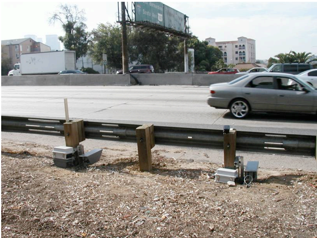
Figure 9 Dual AxleLight Units Set Up to Perform Vehicle Classification Counts
