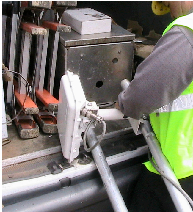
Figure 17 One-Person Setup, Step 1: Attaching Sensor
