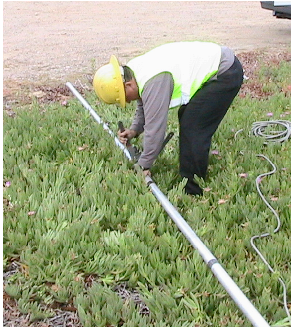
Figure 18 One_Person Setup, Step 2: Connecting Poles
