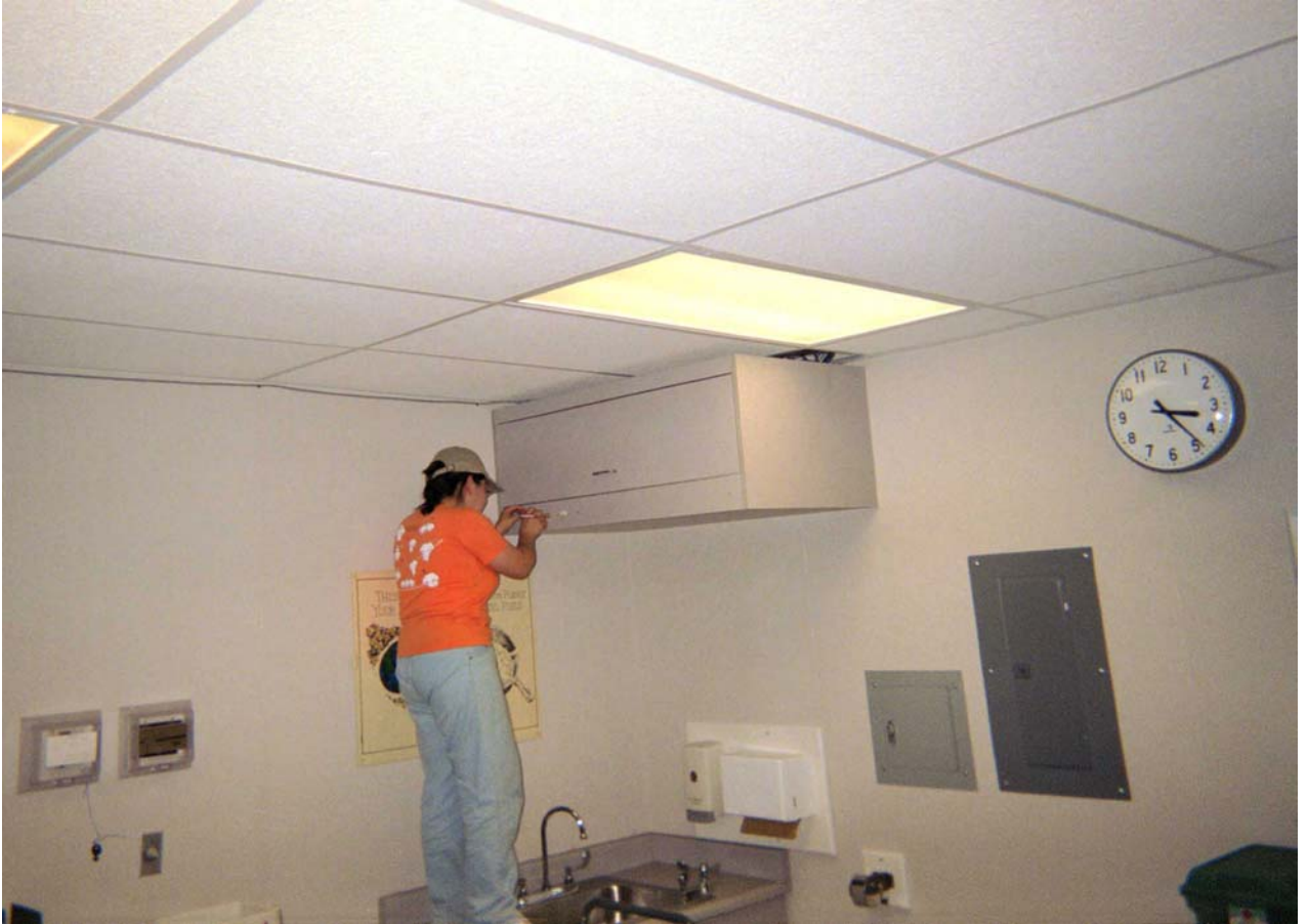
Figure 15: Photograph of LBNL technician placing indoor VOC and aldehyde samples.
