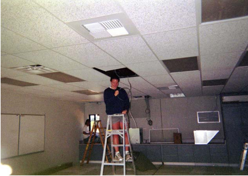
Figure 17 (a-c): Photographs of LBNL designed Lexan mobile located at the center of each RC 1-2 ft down from ceiling, i.e., 6.5 ft above carpeted floor, for SLM (noise level, dB (A)), T and RH measurements, including (a) installation, (b) SLM calibration and (c) co-located Quest M-27 noise dosimeters to validate the orientation and location of the SLM microphone.
