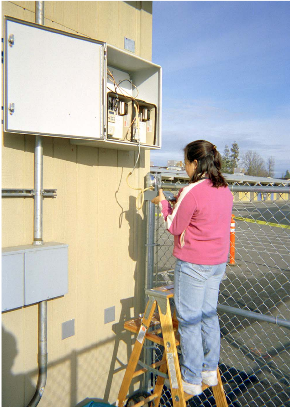
Figure 16: Photograph of LBNL technician conducting flow rate measurements of the aldehyde sampling system with a BIOS DryCal low flow cell calibrator. VOC sampling system flow rates were taken nearby with a simple bubble tube protocol.
