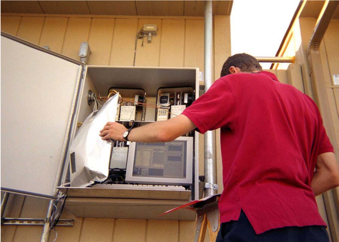
Figure 12: Photograph of LBNL technician conducting calibration protocol for CAI ZFP-9 CO 2 gas analyzers with calibration bags at percentages of 2788 ppm.
