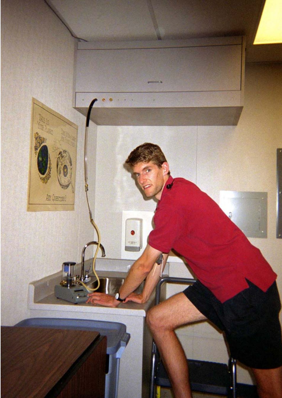
Figure 13: Photograph of LBNL technician conducting flow rate measurements of the PSI MetOne 237B particle counters with a BIOS DryCal low flow cell calibrator.
