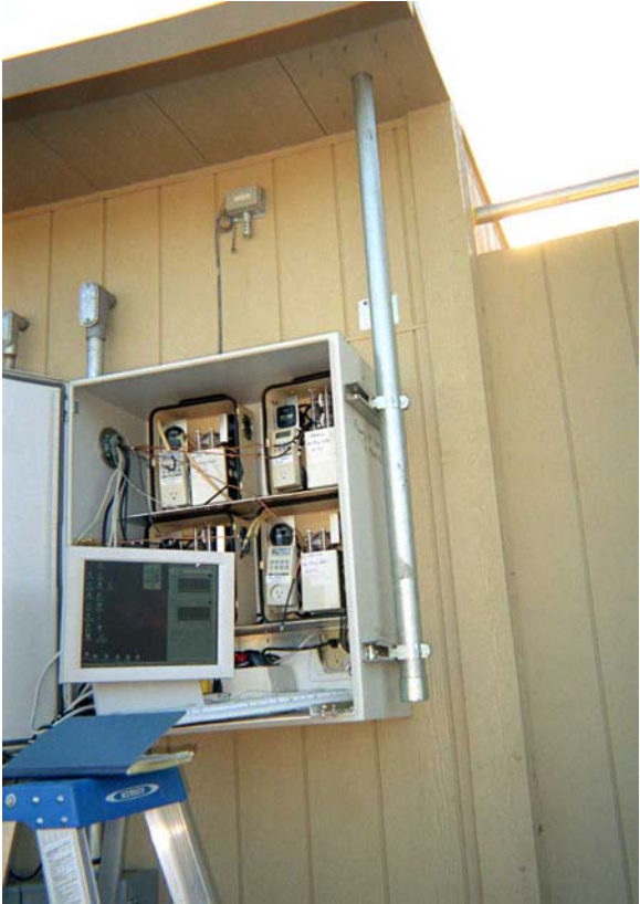
Figure 14 (a-b): Photograph of LBNL outdoor enclosure with (a) VOC and aldehyde sampling systems and (b) sampling lines for outdoor samples.
