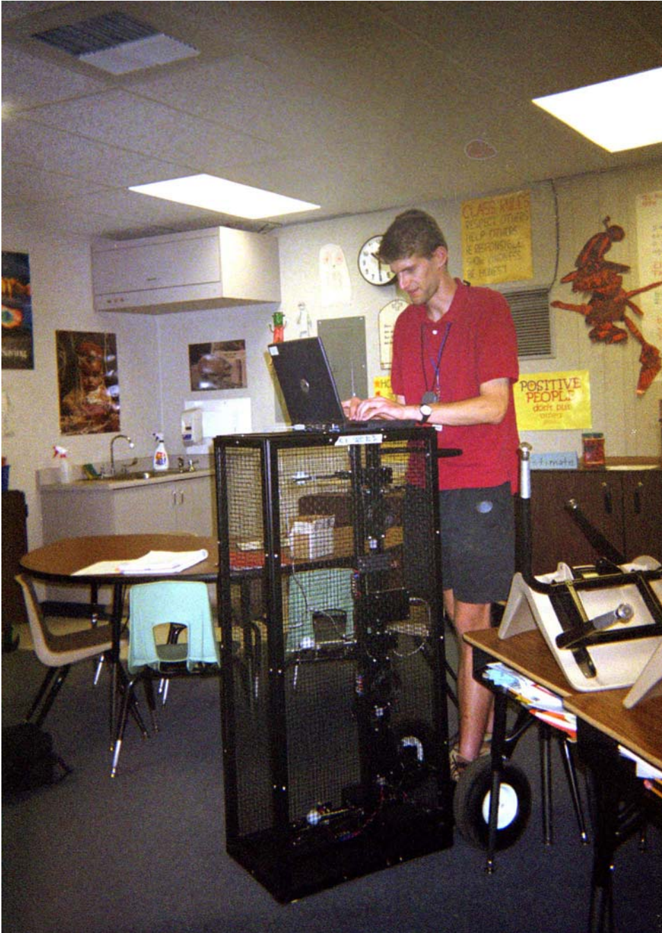
Figure 19: LBNL technician was operating the thermal comfort monitoring cart to power on and off and to download, save, and review data.
