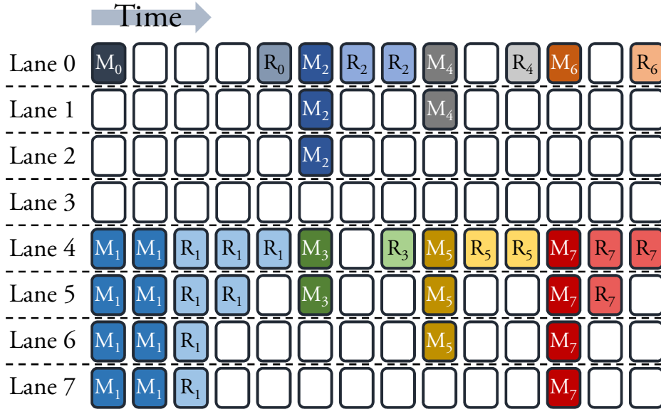
Figure 4.17: Warp execution visualization in sub-warp decomposition (with width 4) for the example in Figure 4.16. Sub-warp decomposition attempts to exploit parallelism inside coarse-grained tasks.
