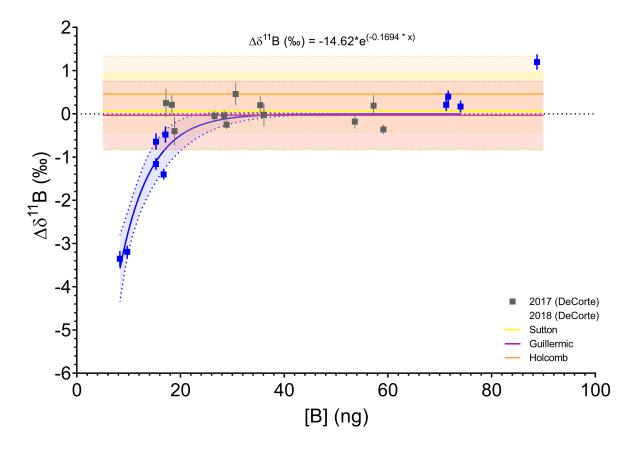
Figure 6.2 NEP standard curve correction for the 2018 samples. There is a clear mass-based correlation to  $\delta^{11}$ B (‰) for the NEP standards. The offset from the 2017 average boron value is defined by the logarithmic relationship:  $\Delta\delta^{11}$ B (‰) = 3.139\*log(x) + 5.342, and has an R<sup>2</sup> value of 0.74.
