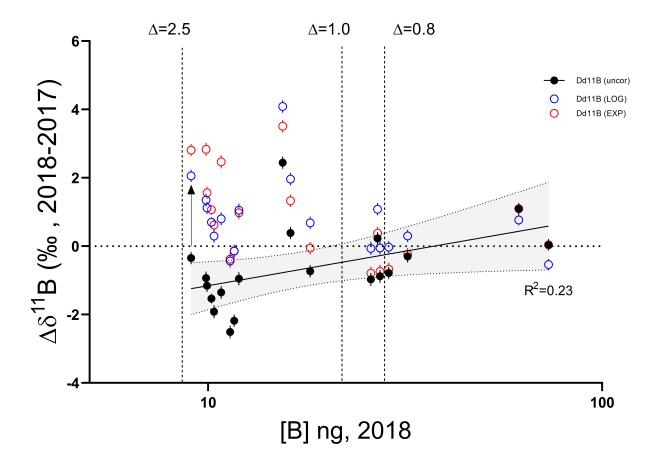
Figure 6.3 NEP standard curve correction for the 2018 samples. There is a clear mass-based correlation to  $\delta^{11}$ B (‰) for the NEP standards. The offset from the 2017 average boron value is defined by the logarithmic relationship:  $\Delta\delta^{11}$ B (‰) = 3.139\*log(x) + 5.342, and has an R<sup>2</sup> value of 0.74.
