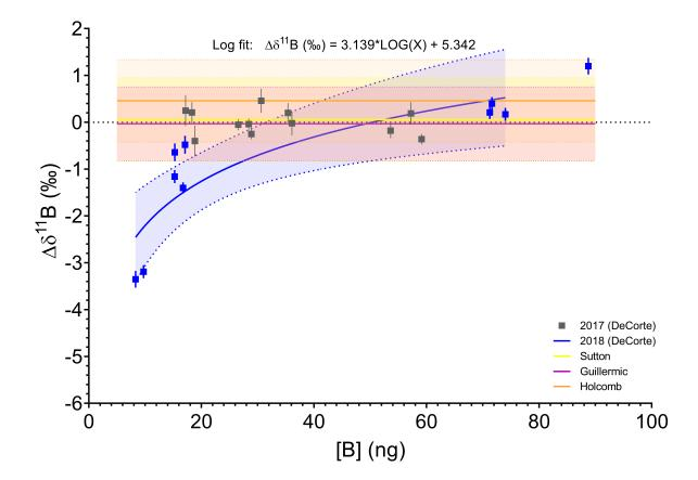
Figure 6.1 NEP standard curve correction for the 2018 samples. There is a clear mass-based correlation to  $\delta^{11}B$  (‰) for the NEP standards. The offset from the 2017 average boron value is defined by the logarithmic relationship:  $\Delta\delta^{11}B$  (‰) = 3.139\*log(x) + 5.342, and has an R<sup>2</sup> value of 0.74.
