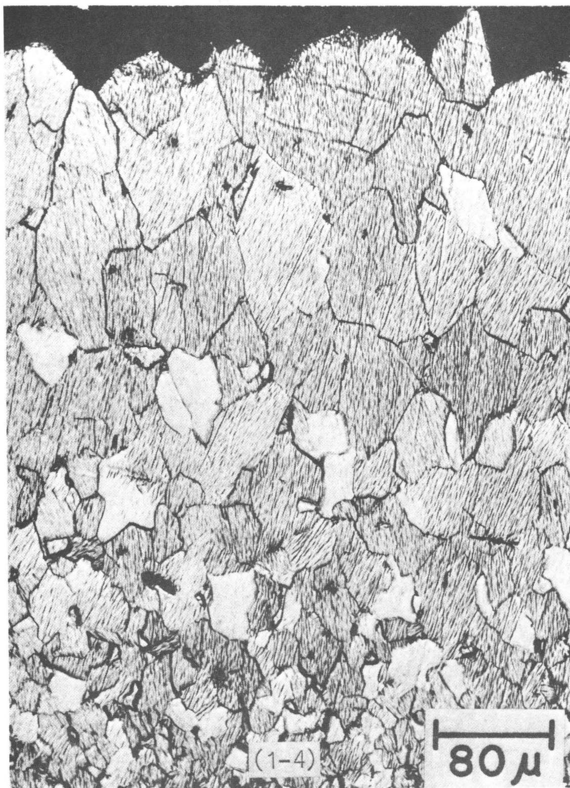
Figure 20. Etched cross section of copper deposit from Ref. 8.
