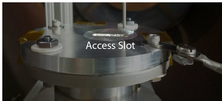
Figure 3.4: Slot cut into cathode surface for Langmuir probe access.
