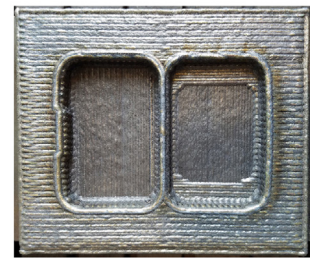
Fig. 8. Grid mold after cladding.
