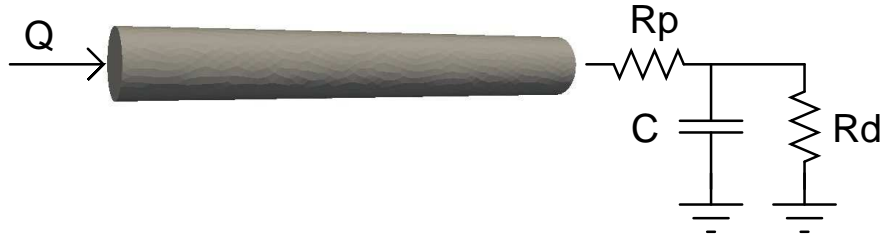
Figure 2.6: Windkessel model coupled to a cylinder with an uncoupled Dirichlet inlet BC. The cylinder diameter and length are 4.0 and 30.0 cm, respectively.
