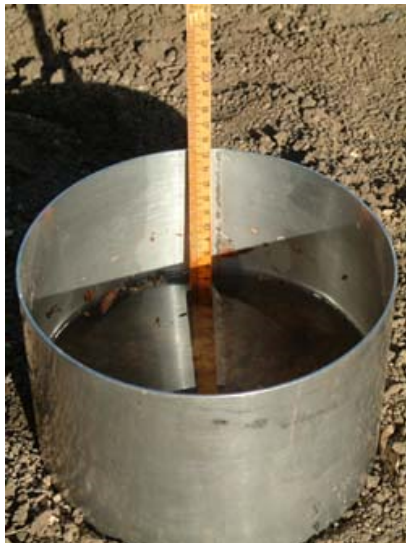
Figure 1. Single-ring infiltrometer, under falling head
