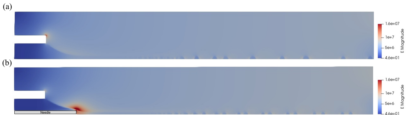
Figure 4.28: Electric field magnitude for (a) the standard emitter and (b) the coaxial emitter at \delta = 2.7 and B_E = 169 .
