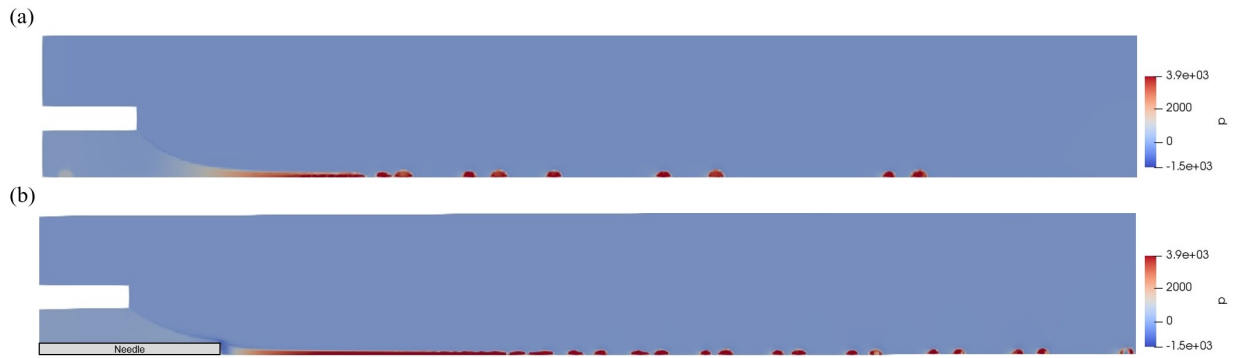
Figure 4.30: Pressure field for (a) the standard emitter and (b) the coaxial emitter at \delta = 2.7 and B_E = 169 .
