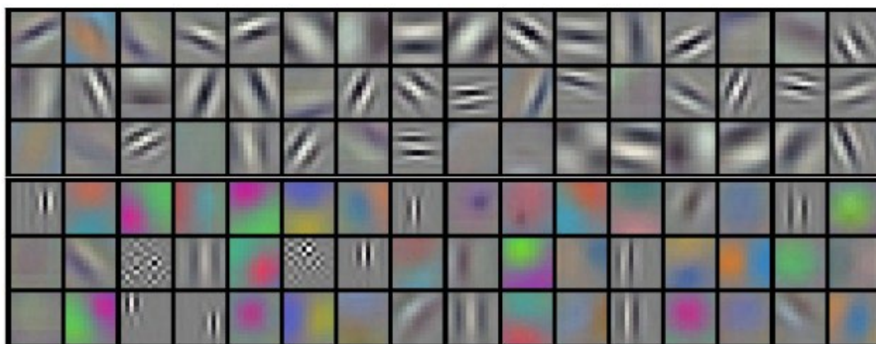
Figure 2.10 Kernels learned by AlexNet [81]. These filters represent image features learned by the convolutional layers. Most were frequency- and orientation-focused.
