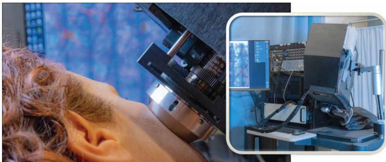
Figure 1. FLAME, a compact and portable multiphoton microscope-based imaging platform, incorporating the Carmel X-780 laser and highly optimized for noninvasive clinical skin imaging. The platform was designed and developed at the Beckman Laser Institute & Medical Clinic at the University of California, Irvine. Photos by Paul Kennedy.
