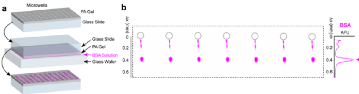
Figure 3: Determination of the technical variation threshold of the microfluidic immunoblot. (a) Schematic of purified protein immunoblotting assay. The polyacrylamide (PA) gel of the microfluidic immunoblotting device is incubated with a solution of fluorescently-labeled bovine serum albumin (BSA) for 30 min for BSA to partition into microwells. Assay is then run as described in main text. (b) False-colored fluorescence micrograph of resulting BSA immunoblots and corresponding fluorescence intensity profiles used to perform area-under-the-curve (AUC) quantification. The coefficient of variation (CV%) was calculated as \text{S.D.}/\text{mean} \times 100 for N = 9 replicates. The technical variation threshold was computed as the mean CV (4.7%) plus three standard deviations for a 99% confidence interval (S.D. = 0.9%) for a CV threshold of 7.4%.
